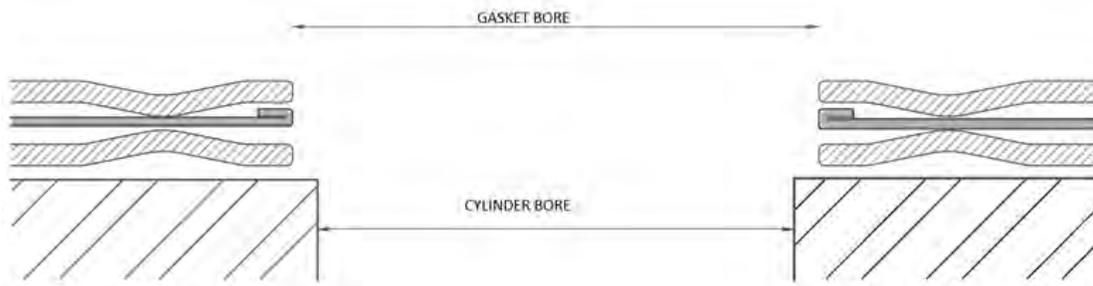
**Note:** Head gasket bore opening should always be larger than the cylinder bore opening. Image depicts Gas Stopper design (MLS GS) head gasket.
