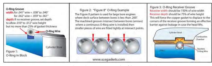
Note: For best results SCE Pro Copper Series (P prefix) Copper Head Gaskets should be used with sealant (if liquid cooled use Copper Coat, SCE p/n G1612) and o-ringed block or heads.
